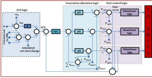
Figure 6: Block diagram of AGC
