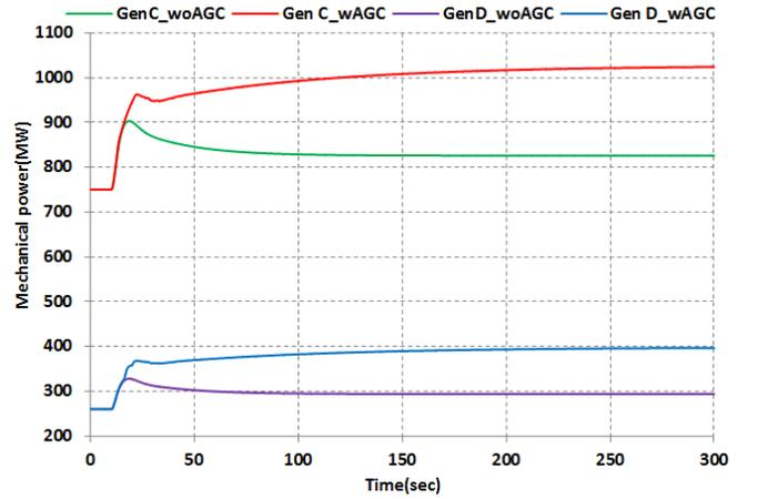
Figure 9: Mechanical input to of the unit C and D under loading less than the maximum generation limit.
