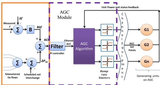
Figure 10: AGC configuration during pilot [4]
