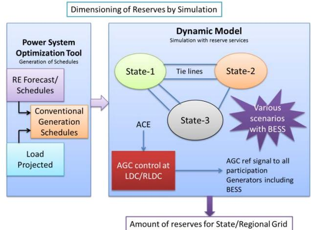
Figure 5: Transient model for secondary reserves calculation
