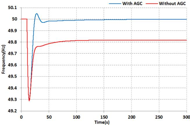
Figure 8: Frequency response with and without AGC under loading less than maximum generation limit
