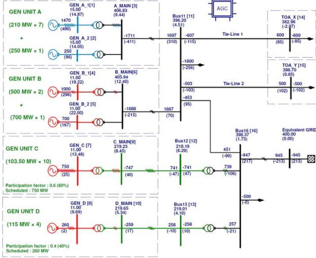
Figure 7: Typical two area system simulated in MiPower [6]
